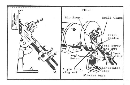
(7) Without altering feed screw position rotate drill bit to engage the other flute. Switch on machine and grind in short sweeps to avoid overheating.
